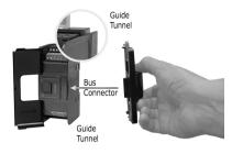
The Base and End Units of the Short-range and Long-range models are **not interchangeable**, do not mix between them.
